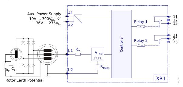
Figure 3.1: Measuring principle of the earth current. C<sub>E</sub> and R<sub>E</sub> are equivalent circuit symbols for the field-to-earth capacitance and resistance, respectively.
