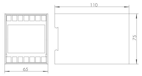
Figure 5.1: Dimensional drawing. (All dimensions in millimeters.)
