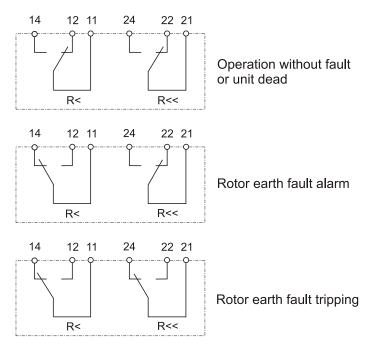
Figure 2.2: Contact positions of the output relays
