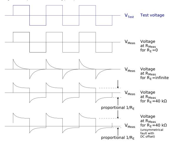
Figure 3.2: Measuring principle
